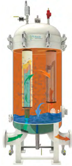
Vertical Two-Stage Coalescer Separator Flow Diagram
